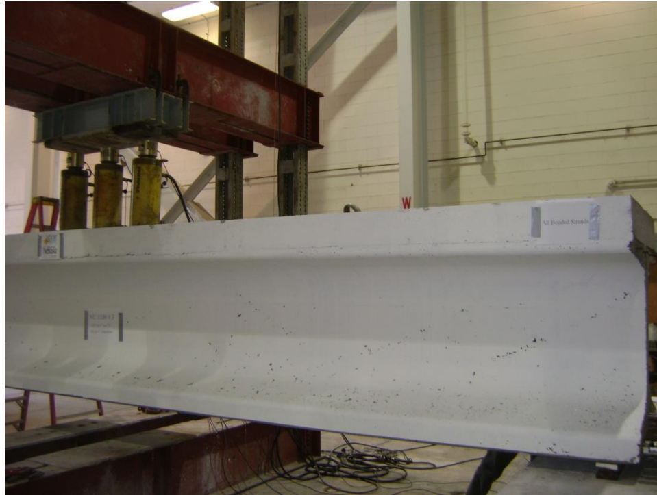
Figure 3.27 NU1100 Development Length Test Setup
