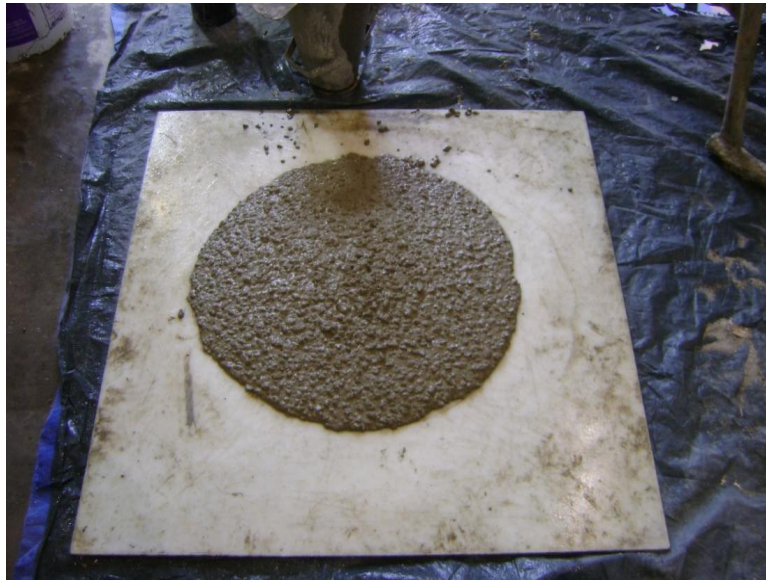
Figure 3.8 T24 Concrete Spread
