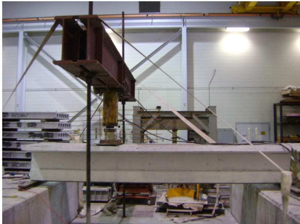
Figure 3.16 T24 Vertical Shear Test Setup
