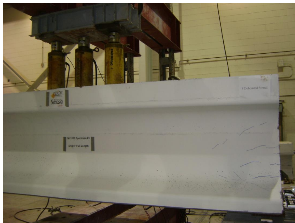
Figure 3.30 NU1100 Vertical Shear Test Setup
